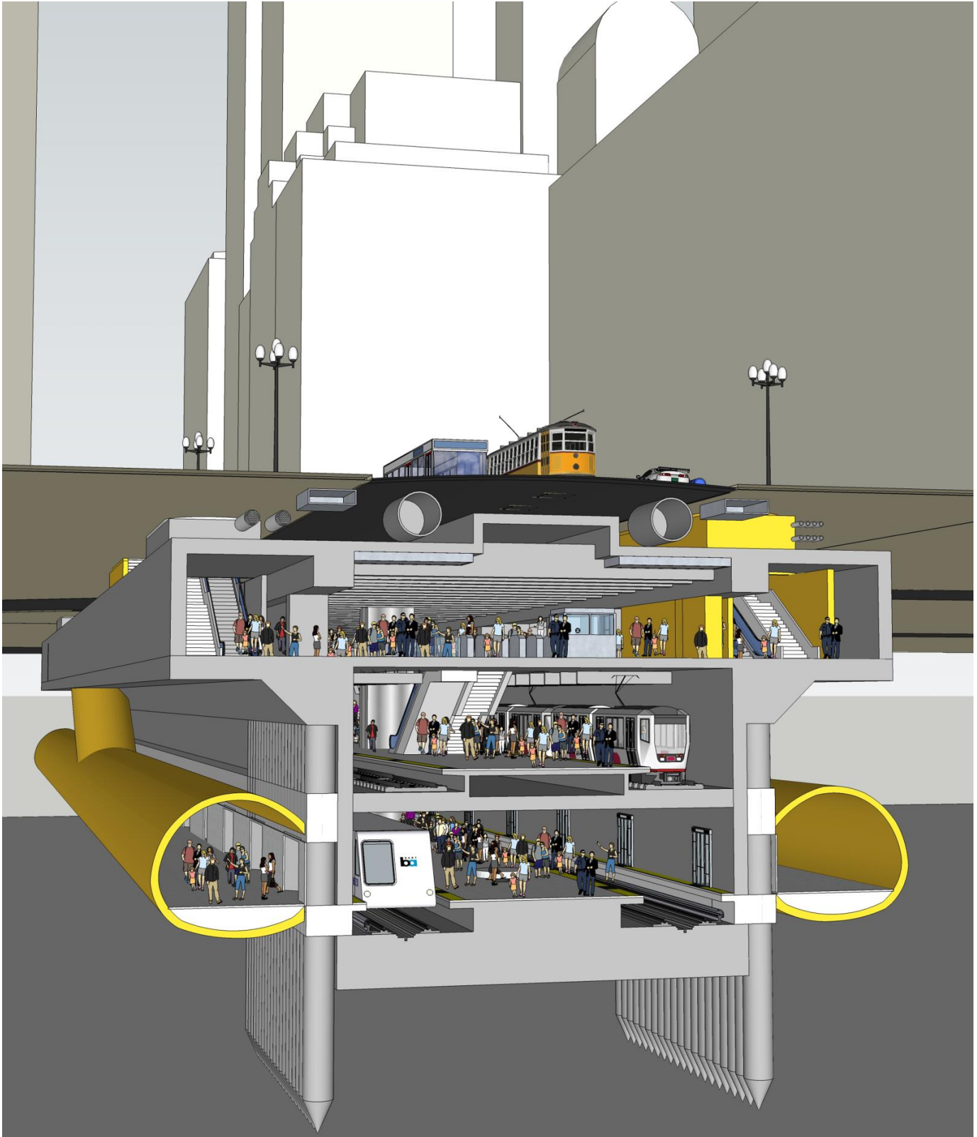
Figure 31: Constructability and Construction Staging Analysis – Side Platforms Study Reflecting mined tunnel construction technique
